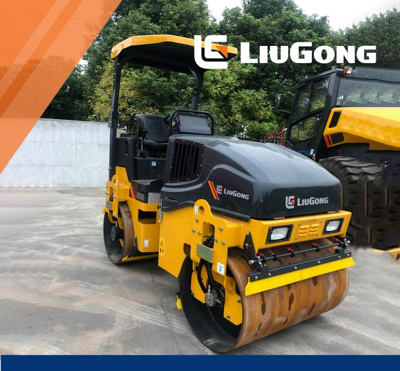
Engine Rated Power Nominal Amplitude Range Vibration Frequency Range Centrifugal Force Range Working Width Operating Weight Perkins 403D-15T 30 kW @ 3,000 rpm 0.35/0.45 mm 60/45 Hz 30/45 kN 1,300 mm 3,500 kg
