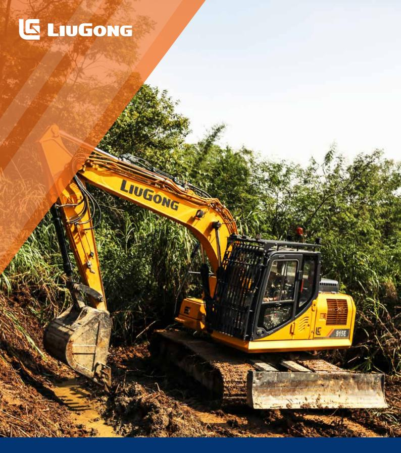
Engine Cummins QSB4.5 Rated Power 90 kW (121 hp / 122 ps) @ 2,200 rpm Net Power 84.3 kW (113 hp / 115 ps) @ 2,200 rpm Maximum Dig Depth 5,470 mm Standard Bucket Capacity 0.6 m $^3$  Operating Weight 15,400 kg
