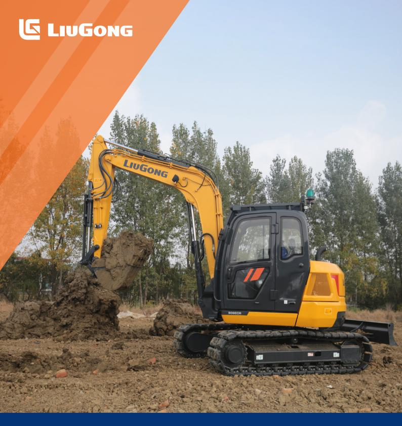
Engine Yanmar 4TNV98C-SLY Rated Power 46.2 kW (62 hp / 63 ps) @ 2,200 rpm Net Power 44 kW (59 hp / 60 ps) @ 2,200 rpm Maximum Dig Depth 4,540 mm Standard Bucket Capacity  $0.28 \text{ m}^3$  Operating Weight 8,700 kg
